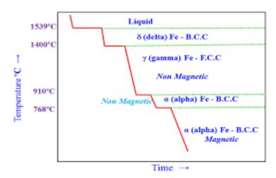
On further cooling at 1400°C, a phase change occurs and the atoms rearrange themselves into (gamma) form which is F.C.C. and non-magnetic. On still further cooling at 910°C, another phase change occurs from F.C.C. non magnetic iron to B.C.C. non magnetic (alpha) iron. Finally at 768°C, the alpha – iron (B.C.C.) becomes magnetic without a change in lattice structure.
