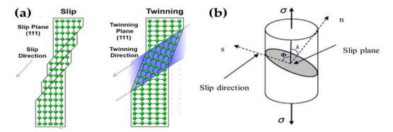
Slip is defined as the process or mechanism by which a large displacement of one part of the crystal relative to another along particular crystallographic planes takes place.
