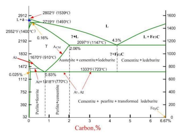
At all temperatures, the following reaction takes place: Fe3C cooling 3Fe + C (graphite) At higher temperatures, the graphitization of the iron- carbide occurs.
