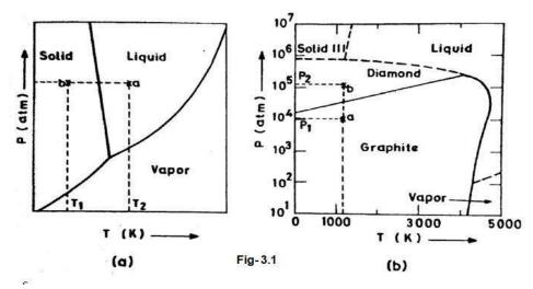
Phase diagrams of two one component system, H2O and carbon as a function of temperature and pressure. In a single-phase region both P and T may be independently varies.
