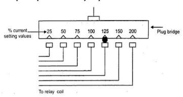
Example: Suppose that an overcurrent relay having current setting of 125% is connected to supply circuit through a CT of 400/5. Find pick-up current.
