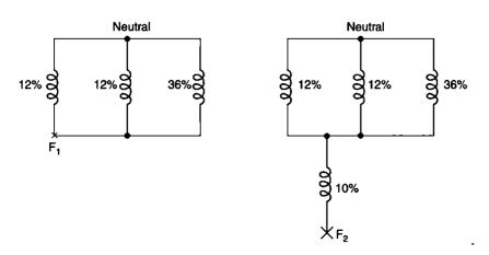
(ii) When the fault occurs on the high voltage side of the transformer (point  $F_2$  in Fig. 1), the reactance diagram will be as shown in Fig. 3.
