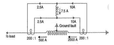
$\triangleright$  If current flows to the fault from both sides as shown in below diagram, then the sum of CT secondary currents i.e 10+5=15 A will flow through the relay.
