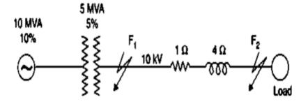
**Solution.** In fig. shows the single line diagram of the network. Let 10,000 kVA be the base kVA
