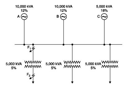
total reactance up to the point of fault  $F_1$  is the parallel combination of the reactances of the three alternators i.e.
