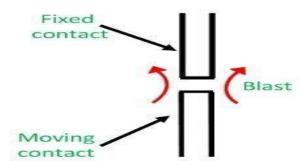
Here the air blast directed along the arc path.
