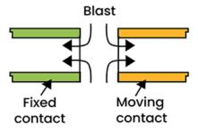
Here the air-blast is directed radially to the arc path.
