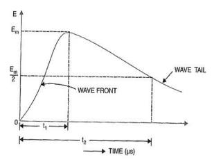
Above figure shows the wave form of a typical lightning surge.
