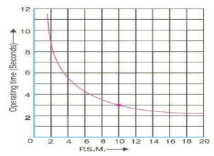
**Example:** Determine the time of a 5-ampere ,3-second overcurrent relay having a current of 125 % and a time setting multiplier of 0.6 connected to supply circuit through a 400/5 current transformer when the circuit carries a fault current of 4000 A. Use the curve as shown in fig.
