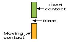
Here the air blast is directed at right angles to the arc path.
