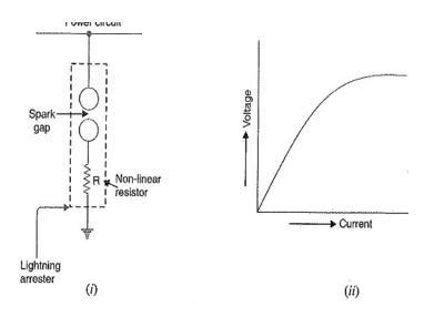
Above figure shows the basic form of a surge diverter.
