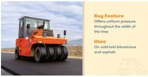
**<u>Pneumatic rollers</u>**, sometimes called pneumatic tyred rollers, are a type of large, ride-on roller with several rows of rubber tires on the front or rear end. The rubber tires provide an 80% coverage area and uniform pressure throughout the width of the tires.
