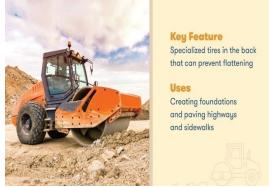
Three-wheeled or single drum rollers are some of the most common pieces of heavy-duty machinery. When people think of road rollers, they typically picture a three-wheeled roller. They typically have a steel drum in the front and two special wheels in the back that can prevent most flat tires from happening.
