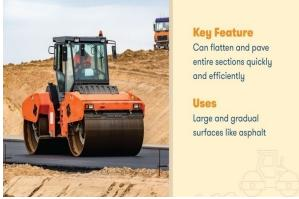
The tandem, or double drum roller, has one steel drum in the front and one in the back. As the two drums move, this moves the roller. The efficiency of the tandem roller comes from the two drums — entire sections of a highway can be flattened and paved quickly and efficiently. These rollers are great for flat or gradual surfaces like asphalt, but because they have very little traction, they're not recommended for anything specialized. Single Drum or Three-wheeled
