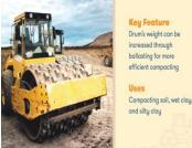
**Sheepsfoot rollers**, otherwise known as padfoot or tamping rollers, are rollers with many rectangular-shaped lugs, or "feet." They're great for compacting soil and silty clay in road construction work.
