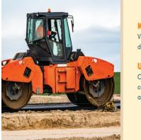
Key Feature Vibrating feature compacts deep under the surface
